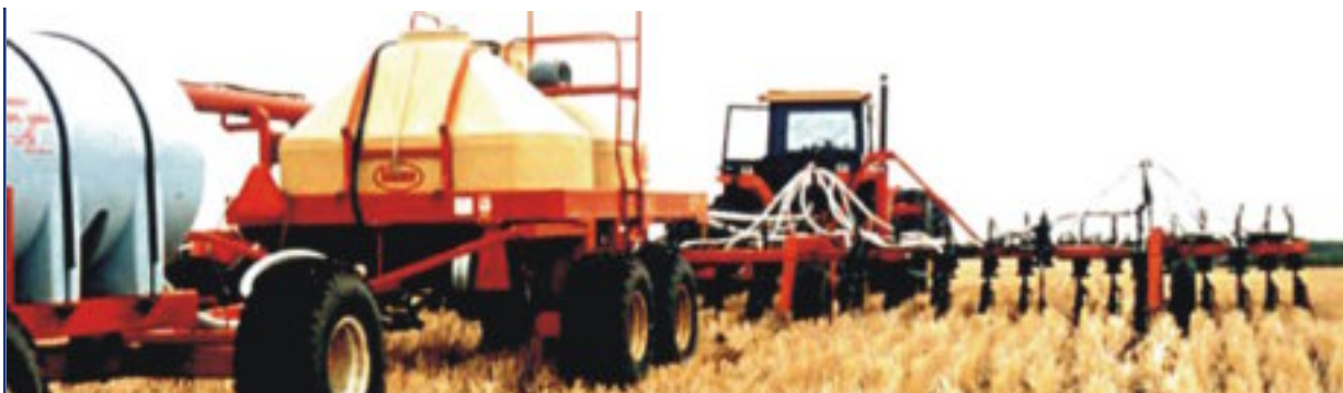
Seeding equipment modified for fluid fertiliser injection
