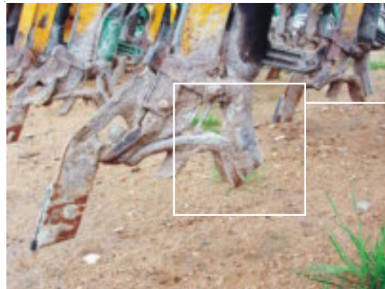
Tyne assembly showing fluid fertiliser injection tube.
